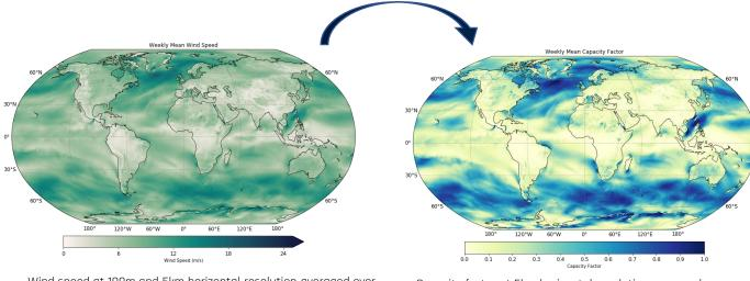
Wind speed at 100m and 5km horizontal resolution averaged over one week in November 2022 (11/11 to 18/11), from 1 hourly wind components (100u, 100v). Data was obtained from the ClimateDT IFS-FESOM production simulation in Marenostrum5. Credit: BSC.
